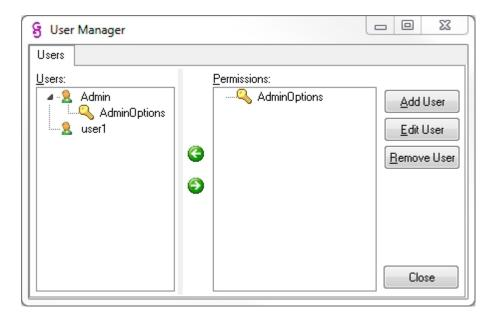
Add or Edit user details using the assigned buttons Admin login cannot be changed with the exception for the password and Full Name
